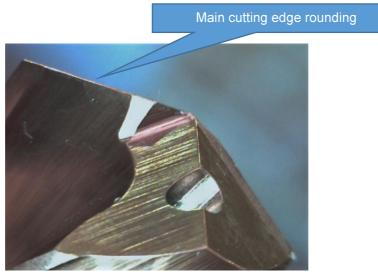
The main cutting edge rounding (for new tools and regrinded tools) is measured using a 3D measuring microscope from Alicona.
