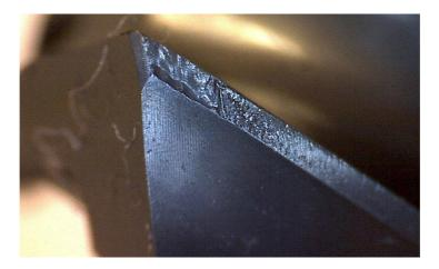
In the case of increased round grinding bevel wear on the outside diameter, the following problems usually occur:
