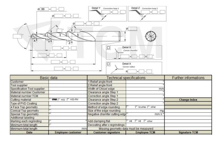
Particular attention must be paid to the rounding of the main cutting edges and the coating of the drills. These data are also stored in the regrinding instructions.
